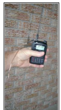
Portable with ¼ whip and counterpoise attached.
