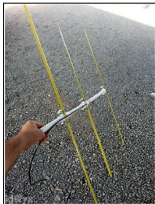
Picture of a hand-held directional 3 element Yagi antenna for ARDF.
